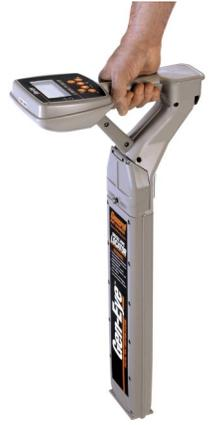
**Tip:** It's much easier to locate the camera when it's closer to the drain opening than when it's 100 feet away. Push the camera five or ten feet into the line, then do your first location. Mark the spot and push the camera ahead another five or ten feet, then repeat. When you're done, you'll have the whole line traced and marked.
