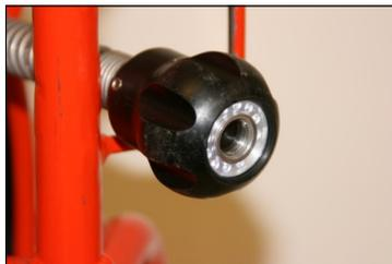
Under normal operating situations, the camera is used with the smaller protective sleeve in 4" lines .
